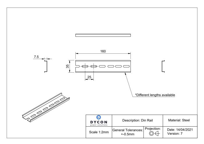
Dycon DIN-rail sections have a standard DIN-rail 'Top Hat' and G profile and are designed to fit in the base of most Dycon housings. They allow you to install any 3<sup>rd</sup> party electrical peripherals that have standard NS32-G & N35 7.5/15mm DIN-rail mountings. The Dycon E-box has ready-drilled holes for a DIN-rail to be fitted and can be supplied with a suitable DIN-rail already in position.
